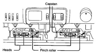
It is recommended that the head assembly be demagnetized if distortion or poor sound quality persists after cleaning the heads. Demagnetize them using a demagnetizer available from an audio store.
