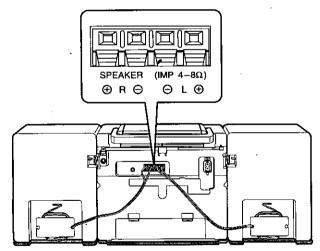
When using the unit with the speakers attached, wind the speaker cables as shown.
