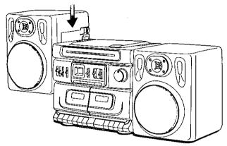
Connect the speaker cable (black) to the  $\Theta$  (negative) speaker terminal, and the other speaker cable (red) to the  $\Theta$  (positive) speaker terminal.
